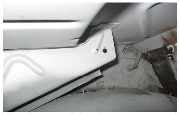
5. With the struts facing the center of the car, slide the hinge into the pocket strut first. Push ball stud through the 5/16" hole, and secure with a washer and nut. Install the new hinge pins and bend the tab back down.6. Reinstall and align the trunk lid using your new hardware.
